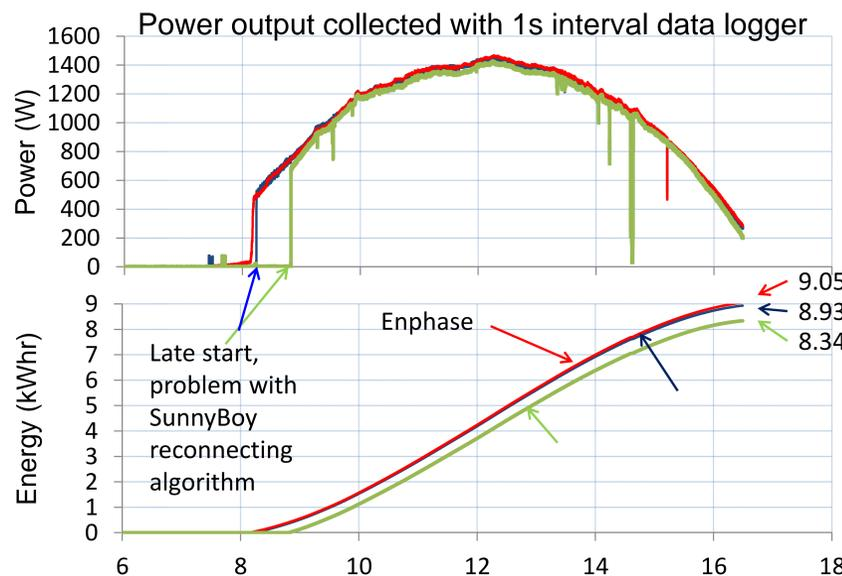
Late start showing significant energy production deficiency with the Sunnyboy inverter design
